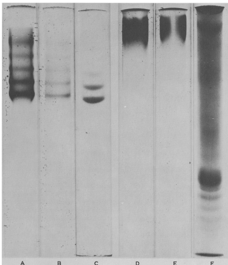
Fig. 3. Polyacrylamide gel patterns of concentrated LDH activity-containing fractions. A, B, C = pooled second (eluant without NADP); LDH activity peak; D, E, F = pooled first peak. A and D-lactate staining; B and E = OH-valeric acid staining; C and F = protein stain (Coomassie blue).
